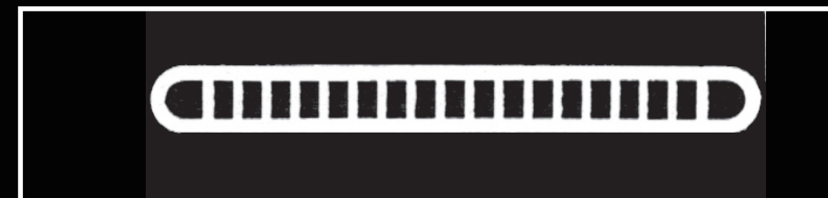
Cross-section of condenser tube
