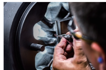
High-quality extruded shapes at UACJ Whitehall are produced using state-of-the-art presses and expertly crafted dies.
