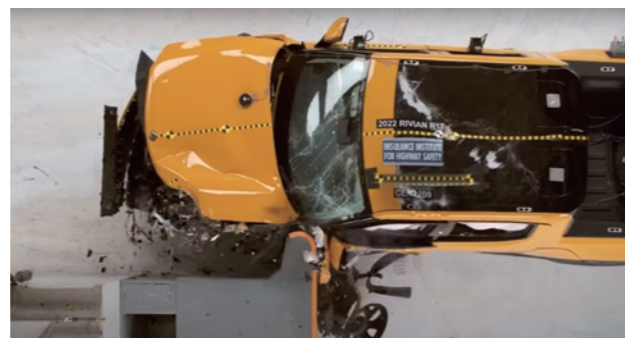
2022 Rivian R1T drive-side small overlap front IIHS crash test © IIHS
