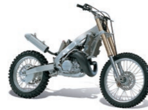
Aluminum extruded products are used to produce motorbike frames and front forks. UACJ's front fork outer tubes hold the world's top share.
