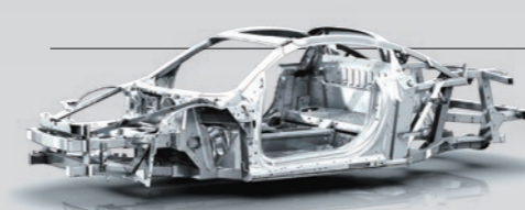
Aluminum alloy space frame | Audi R8
