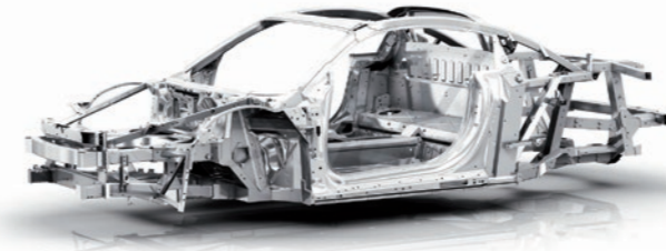
The first-generation Audi R8 was the first mass-market automobile to employ tailored blanking.
