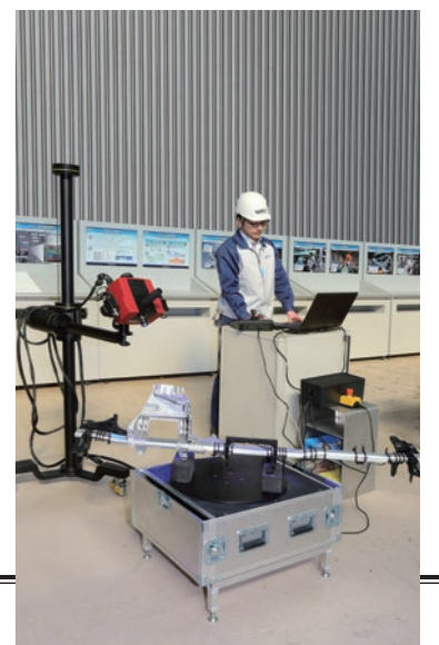
Contactless Coordinate Measuring Machine: Measures the cross-sectional shapes, etc., of automotive parts
