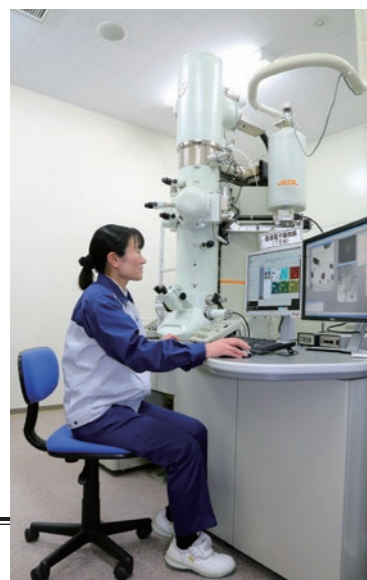
Field-Emission Transmission Electron Microscopy (FE-TEM): Observation and analysis of the crystal structure of aluminum materials
