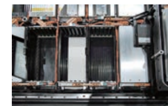
The large-capacity lithium-ion battery loaded on the Audi e-tron is made up of aluminum alloy modules, each containing 12 ‘pouch’ cells. To produce the battery pack, the modules are placed in an aluminum alloy housing.
