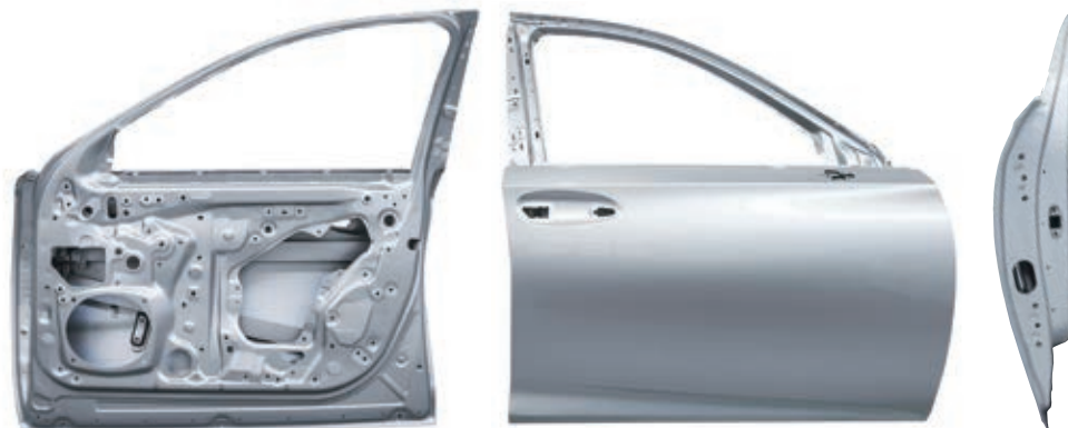
← ↑ This photograph shows how deeply the alloy was drawn to produce this inner door panel. 6000 series aluminum alloys are used for both the inner and outer door panels of the LS.
