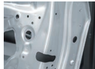
← ↑ This photograph shows how deeply the alloy was drawn to produce this inner door panel. 6000 series aluminum alloys are used for both the inner and outer door panels of the LS.
