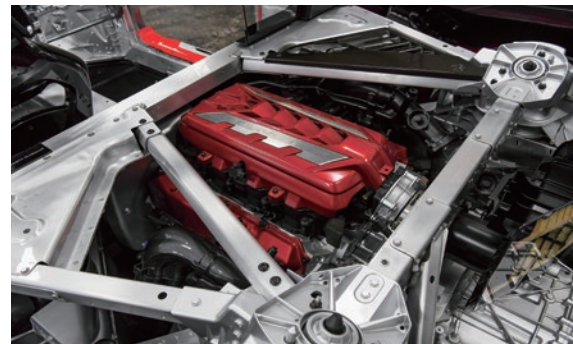
The die-cast aluminium rear shock towers are supported by extruded aluminium reinforcements.
