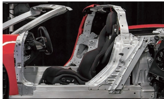
The aluminium stamping parts are joined to the aluminium extruded center pillar using flow-drilling screws.
