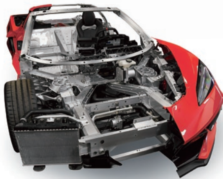
↓ The C8 is a "tunnel-dominant" structure that serves to connect the frame from the front rail to the center tunnel.
