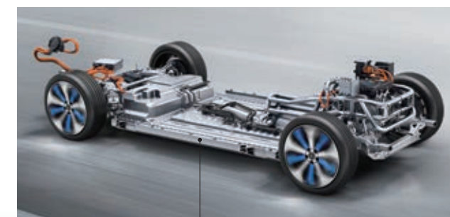
Mercedes-Benz EQC Side impact protection structure (aluminum extrusion)
