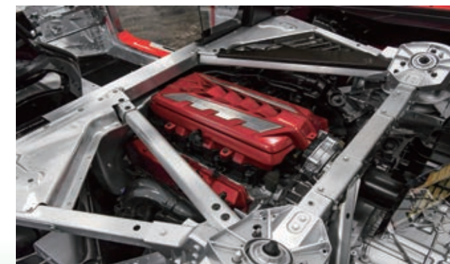
Aluminum alloy extruded shapes (various types of braces)
