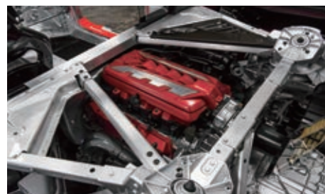
Shock towers are supported by aluminum extruded cross members and braces.
