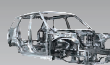
All-aluminum monocoque body > Range Rover Sport
