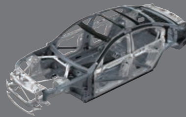
Multi-material monocoque body
