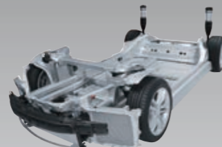
All aluminum alloy platform > TESLA MODEL-S
