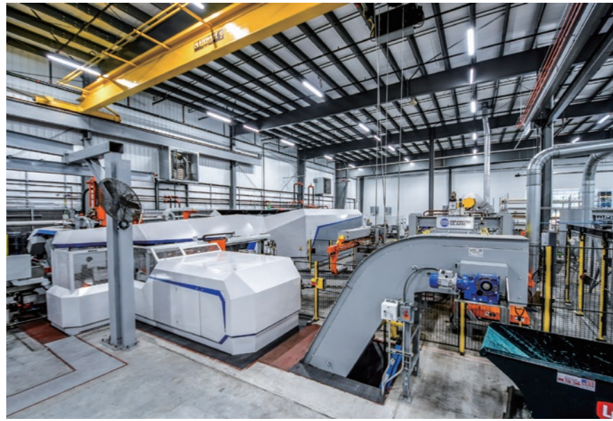
High-Precision Aluminum Alloy Extrusion Press and Cooling Equipment UACJ Automotive Whitehall Industries Manufacturing Department
